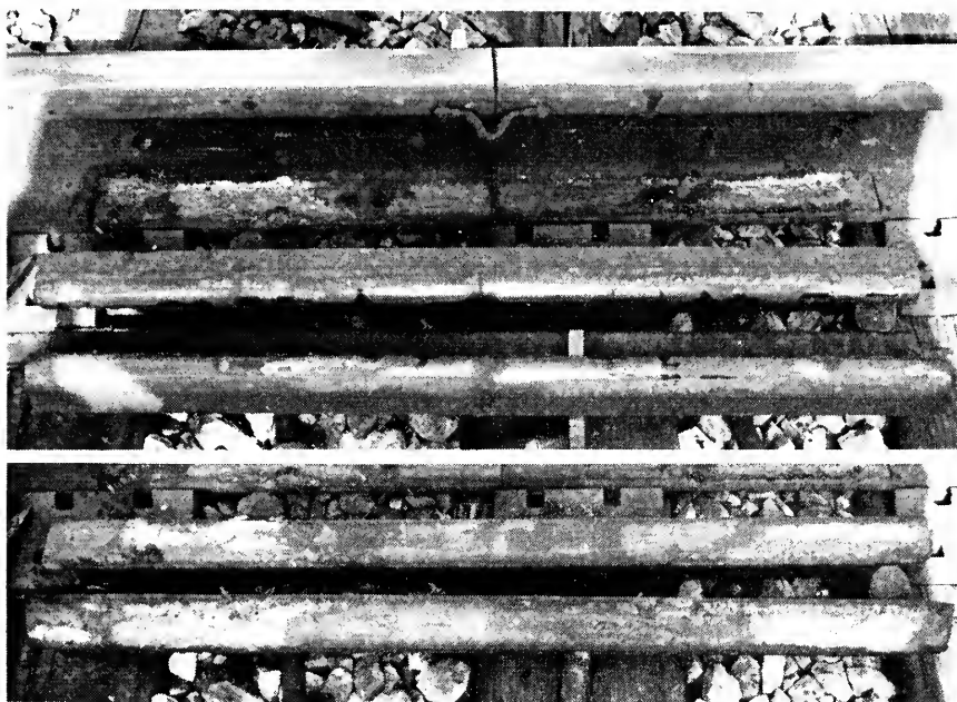
Fig. 16. East Rail Section 7. Spray Coat of Leadolene Barexite No. 690 after One Year of Service.
